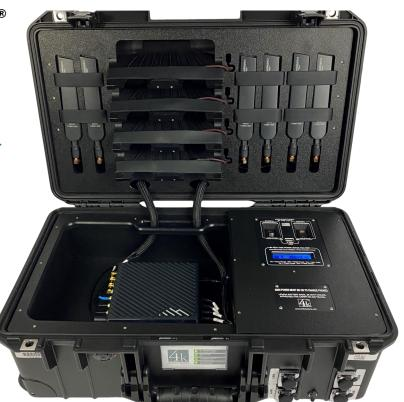
and the Sonim XP8 (smartphones not included). These R1900 modems support worldwide, SIM-based, auto-carrier selection and also available CBRS Band 48 and Band 14. The **MBK Elite** "5G" provides WiFi 6 wireless and gigabyte networking options.
