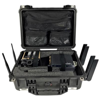
The MBK-1900 FRC "RangerNet™ is designed to utilize external antenna systems.
