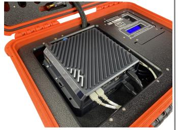
The MBK-1900's integrated Cradlepoint R1900 router is a 5G Embedded High-Performance Solution.
