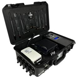
The 4K-MBK-FPS-505H's integrated Cradlepoint R1900 router is a 5G Embedded High-Performance Solution.
